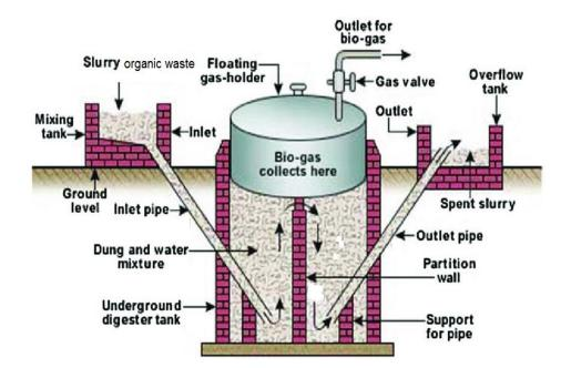
The technical specifications of the modified KVIC model bio-digesters are as follows:
